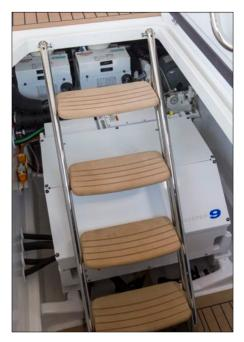
The first yacht with **Seakeeper Gyrostablizer** as standard equipment to stop the roll... a major source of discomfort on all powerboats.
